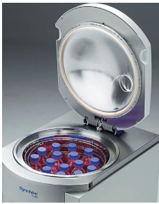
(b) Autoclave used for pre-heat treatment
