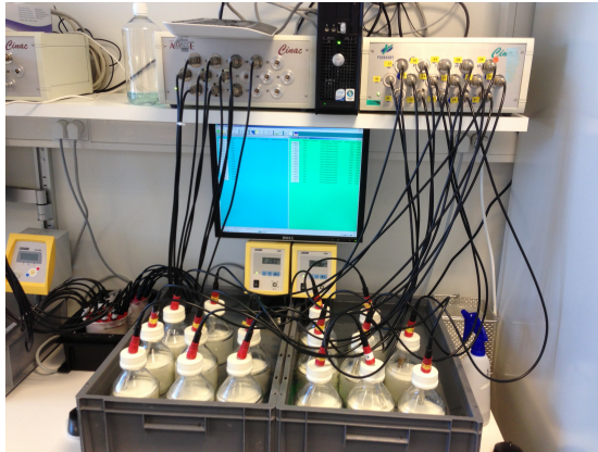
(a) Monitoring the pH development during milk fermentation in two water baths
