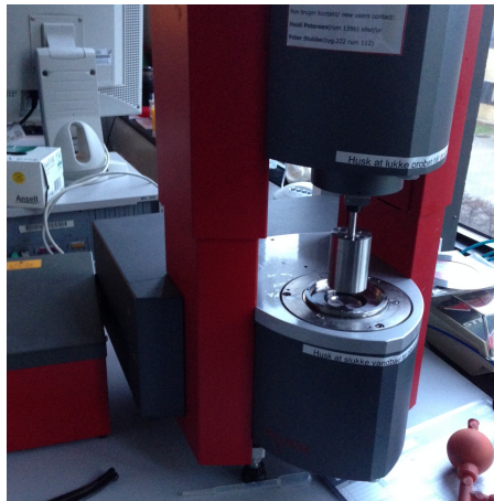
(c) The geometry installed in a rheometer, where it can be lowered to measuring position.
