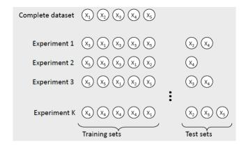
FIGURE 30 GRAPHICAL EXAMPLE OF BOOTSTRAPPING. THE NUMBER OF BOOTSTRAPS (K) IS TYPICALLY SET TO 500.
