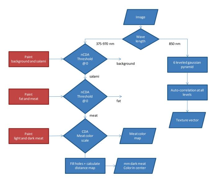
Figure 3 Flowchart illustrating the steps involved in finding and measuring meat colour and salami structure. Left column illustrates the steps involved in measuring colour development, the right column the structure quantification.
