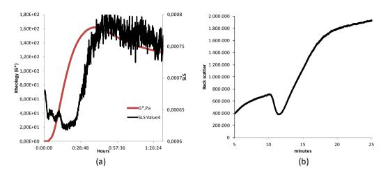
FIGURE 35 EXAMPLES OF PROCESS MONITORING USING SUBSURFACE LASER SCATTERING. (A) MILK ACIDIFICATION FOLLOWED BY RHEOLOGY AND SLS, (B) FAT CRYSTALLISATION (OCCOURING AROUND 10-11½ MINUTES).
