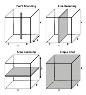
FIGURE 13 APPROACHES FOR CONSTRUCTING SPECTRAL IMAGE CUBES CONTAINING SPATIAL (X AND Y) AND SPECTRAL (λ) INFORMATION. ARROWS REPRESENT SCANNING DIRECTIONS, AND GRAY AREAS REPRESENT DATA ACQUIRED AT A TIME [SUN, 2010].
