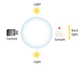
Figure 1. Illustration of instrument setup. A flask with sample is placed at an opening in an integrating sphere. The light source is ten diffuse LEDs and one LED backlight. A multiwavelength image is acquired with a gray tone camera by strobing one LED at a time.
