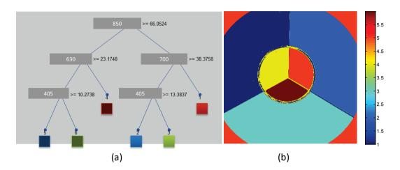
FIGURE 27 DECISION TREE FOR SEPARATING 6 CLASSES OF COLOURED PAPER. (A) TREE MODEL, NUMBER IN DARK BOX SHOWS WHICH WAVELENGTHS TO SPLIT AND AT WHICH VALUE, SEE WAVELENGTHS IN FIGURE 23C, (B) THE RESULTING CLASSIFICATION.
