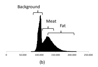
FIGURE 17 SALAMI IMAGE (A) AND CORRESPONDING HISTOGRAM OF GRAY LEVELS (B). MEAT AND FAT SEGMENTATION WITH A GLOBAL THRESHOLD IS NOT POSSIBLE DUE TO THE LARGE OVERLAP IN PIXEL INTENSITIES (DARK EDGE AND LIGHTER CENTER).
