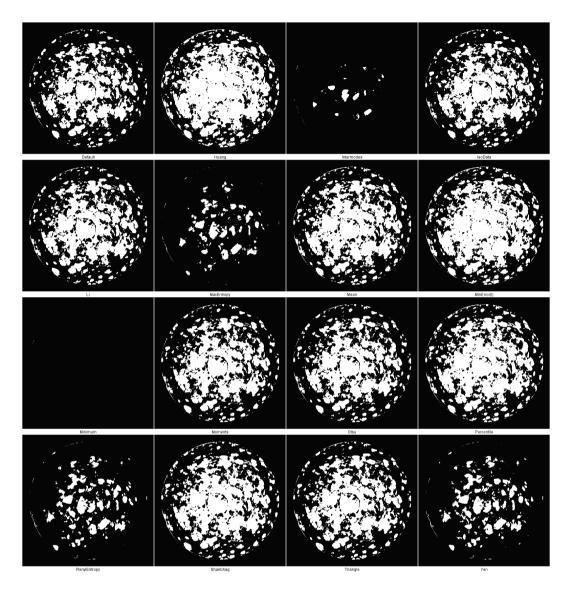
FIGURE 18 25 METHODS FOR AUTOMATIC THRESHOLDING OF GRAY SCALE IMAGES. THE METHODS ARE, <u>ROW 1:</u> DEFAULT(ITERATIVE INTERMEANS, HUANG, INTERMODES, ISODATA, <u>ROW 2:</u> LI, MAXENTROPY, MEAN, MINERROR(I), <u>ROW 3:</u> MINIMUM, MOMENTS, OTSU, PERCENTILE, <u>ROW 4:</u> RENYIENTROPY, SHANBHAG, TRIANGLE AND YEN.
