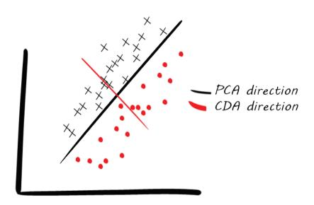
FIGURE 25 AN ILLUSTRATION OF THE FIRST PRINCIPAL COMPONANT AND CANONICAL DIRECTION IN A SIMPLE DATA SET WITH TWO CLASSES OF OBJECTS (X AND \*). THE PCA MAXIMISES THE DATA VARIATION THE PCA MAXIMISES THE CLASS SEPARATION.
