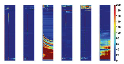
**Figure 6.** H-domes barcodes for the 6 chocolate milks. Each barcode represents 3 days of analysis at 505 nm. The x-axis represents time. Samples 3 and 6 show marbling developing immediately after production.
