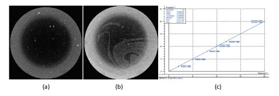
FIGURE 40 COFFEE WHITENER QUALITY AND DEFECTS. (A) FLOCULATED PROTEIN AGGREGATES, (B) FEATHERING, (C) CALIBRATION CURVE TO PREDICT % COFFEE WHITENER IN COFFEE.
