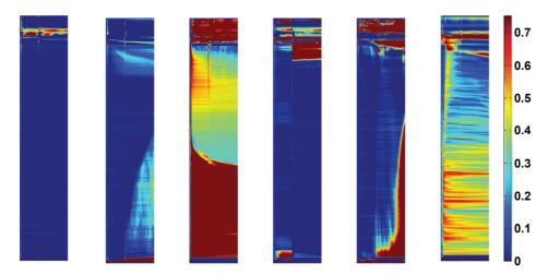
**Figure 7**. Standard deviation barcodes for the 6 chocolate milks. Each barcode represents days of analysis at 505 nm. Blue colors indicate a homogeneous product. A high standard deviation is seen for samples with marbling (samples 3 and 6) and for samples with curdling (samples 2 and 5).
