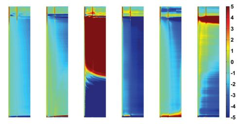
**Figure 5.** Median barcodes for the 6 chocolate milks. Each barcode represents 3 days of analysis at 505 nm. The x-axis represents time. Column points are calculated by a median filter of the original image rows. No change is represented by green, a darker or lighter color by blue and red, respectively.
