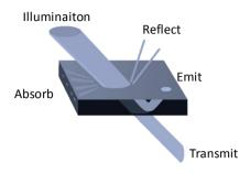
FIGURE 9 ILLUSTRATION OF HOW LIGHT INTERACTS WITH AN OBJECT. LIGHT CAN BE ABSORBED, REFLECTED, EMITED AND TRANSMITTED (MODIFIED FROM [MARTIN, 2011]). SURFACE AND SUBSURFACE PROPERTIES DETERMINES HOW AND HOW MUCH LIGHT IS REFLECTED [SALEH, 2011].
