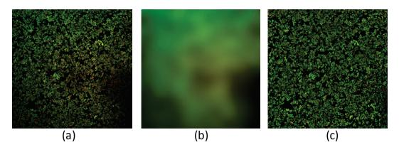
FIGURE 16 CORRECTION OF UNEAVEN ILLUMINATION OF MICROSCOPY IMAGES. (A) ORIGINAL IMAGE DARK AREAS DUE TO POOR STAIN DIFFUSION, (B) GAUSSIAN FILTER OF ORIGINAL IMAGE, (C) CORRECTED IMAGE(A/B). THE CONFOCAL IMAGE IS OF A YOGHURT, PROTEIN IS STAINED GREEN AND FAT IS RED.
