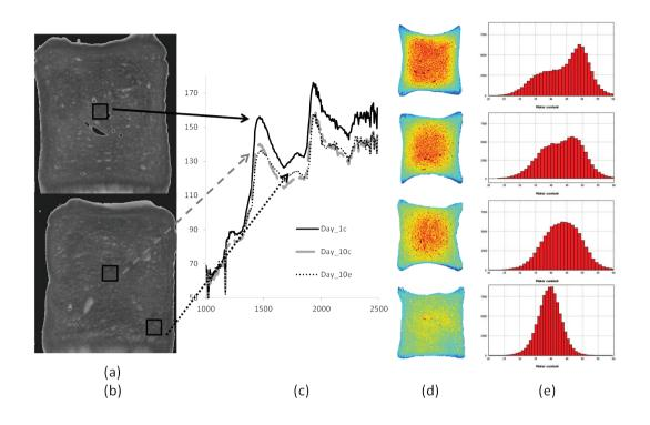
FIGURE 43 HYPERSPECTRAL IMAGES OF WHITE BREAD. (A) DAY 1 BREAD (1300 NM), (B) DAY 11 BREAD (1300 NM), (C) MEAN SPECTRA FROM CENTER OF DAYS 1+11 AND EDGE DAY 10, (D) PREDICTED WATER CONTENT, TOP-TO-BOTTOM: DAYS 1, 4, 7 AND 11, (E) HISTOGRAM OF WATER DISTRUBUTION OF BREAD ON DAYS 1, 4, 7 AND 11.
