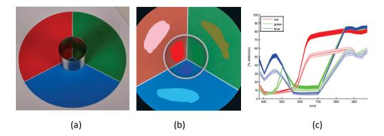
FIGURE 23 RED-GREEN-BLUE PAPER WITH SHADOW IN THE CENTER CAUSED BY METAL CYLINDER: (A) PHOTO OF SET-UP; (B) ANNOTATED VIDEOMETERLAB IMAGE, TWO AREAS FOR EACH COLOUR ARE SELECTED, I.E. INSIDE AND OUTSIDE THE METAL CYLINDER; (C) SPECTRA WITH STANDARD DEVIATION FOR THE 6 ANNOTATED AREAS.
