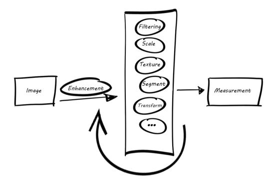
FIGURE 1 POSSIBLE STEPS IN IMAGE ANALYSIS. THE RAW IMAGE DATA IS OFTEN ENHANCED, E.G. FOR NOISE REDUCTION, CROPPING OR CALIBRATION. A TYPICAL IMAGE ANALYSIS NORMALLY COMBINES SEVERAL STEPS OF ANALYSIS, E.G. SEVERAL SEGMENTATIONS CAN BE COMBINED INTO ONE SEGMENTATION. BASED ON ONE OR SEVERAL SEGMENTATIONS CAN RELEVANT IMAGE FEATURES BE MEASURED, E.G. NUMBER OF OBJECTS, TEXTURE, SPECTRAL OR SHAPE.
