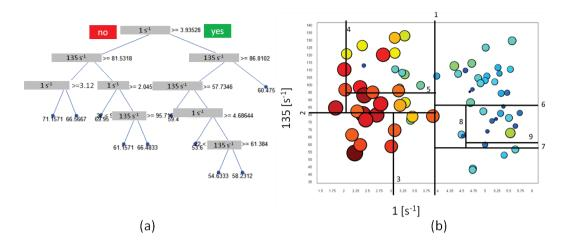
FIGURE 29 YOGHURT SYNERESIS (%) PREDICTED USING TWO VARIABLES (SHEAR STRESS AT 1 AND 135 S<sup>-1</sup> MEASURED BY RHEOLOGY FLOW CURVES). (A) THE REGRESSION TREE – THE PREDICTED VALUE IS SEEN AT THE BOTTOM OF THE LEAVES, (B) SCATTER PLOT OF THE TWO MODEL VARIABLES, THE TREE NODES ARE SHOWN WITH NUMBERED LINES. THE SIZE COLOUR OF SCATTER PLOT POINTS INDICATES LEVEL OF SYNERESIS (%).
