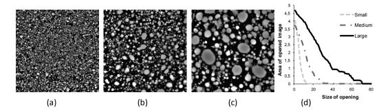
FIGURE 22 CONFOCAL IMAGES OF OIL EMULSIONS AND THEIR CORRESPONDING GRANULOMETIC CURVES. (A) EMULSION WITH SMALL OIL DROPS, (B) MEDIUM SIZED, (C) LARGE OIL AND (D) THE GRANULOMETRIC CURVE.
