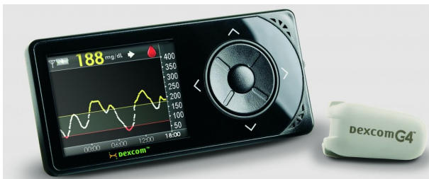
Figure 2.2: The Dexcom G4 ® Continuous Glucose Monitor assist diabetics monitor their blood glucose in real-time [6].
