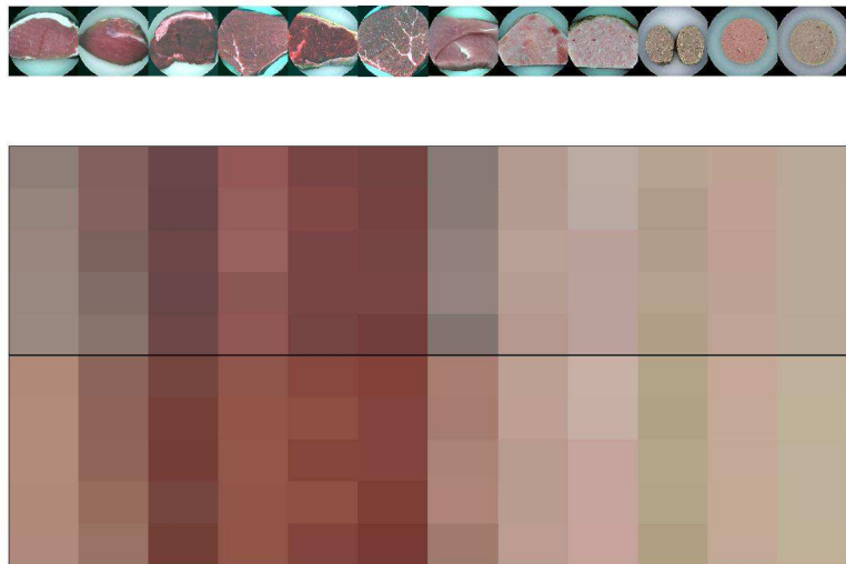
Figure 6: Top row are examples of each of the 12 types of meat considered. These are pseudo RGB images. Bottom rows: Average measurements for the colorimeter and the VideometerLab for the five samples of each type in sRGB.
