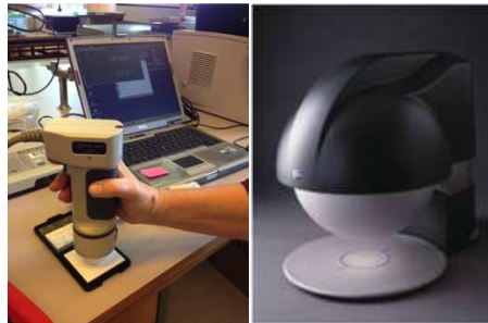
Figure 1: Left: Calibration procedure for the colorimeter Minolta CR-300. Right: The multispectral imaging system VideometerLab.
