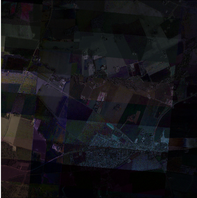
Figure 5.10: The figure shows the numerical difference between the standard deviation images shown in Figure 5.9c and 5.9d, respectively. The values have been multiplied by a factor of 25 in order to make the differences in the images more visible.
