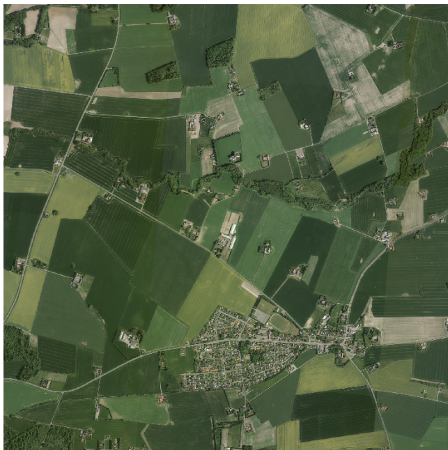
Figure 5.39: The figure shows the result from global gradual matching with the division method using 8-neighbourhood, damping parameters of w_a = w_b = w_c = 0.025 , and boundary conditions with damping parameter w_B = 10 and boundary width \delta = 3 .
