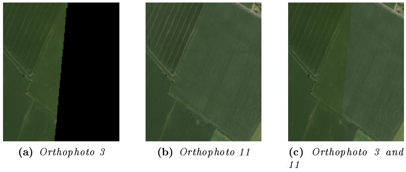
Figure 1.1: The figure shows the seamline between two orthophotos in a small area of the graphical map. The black area in (a) is outside orthophoto 3.
