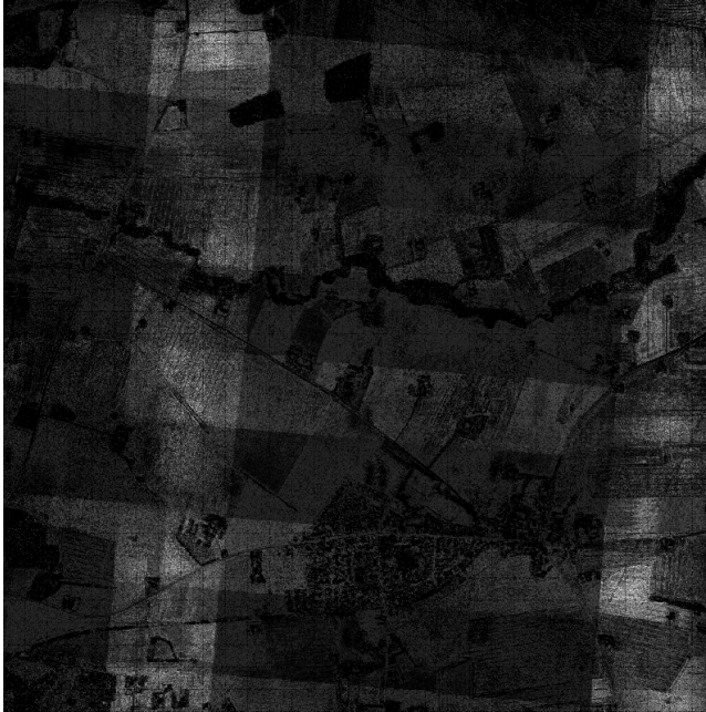
Figure 5.8: The figure shows the final weights calculated in the change detection algorithm for each pair of neighbours using 4-neighbourhood. The dark pixels in each overlap are removed in the final thresholding.
