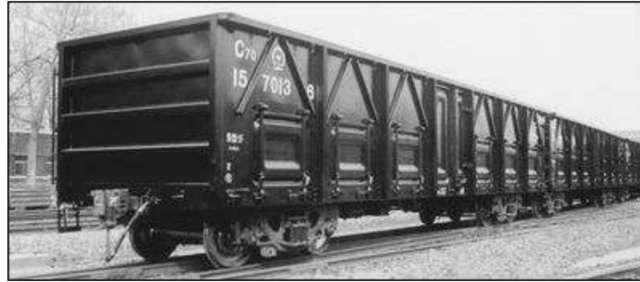
Fig. 7. A 4-axle Chinese hopper wagon.
