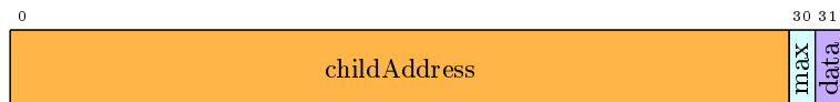
Figure 6.1: NodeChildData is encoded in a 32 bit int. It contains the address of the first child in the node tile, and two flags signaling: if the node is at max subdivision level, and the data type of the volume data associated with the node.
