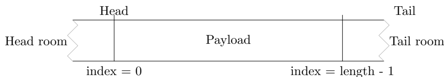
Figure 3.1: packet_data abstraction. The Head and Tail pointers can be moved independently, growing or shrinking the payload area in the given direction.
