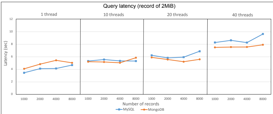
Figure 5.10: Media query latency as a function of the total number of files
