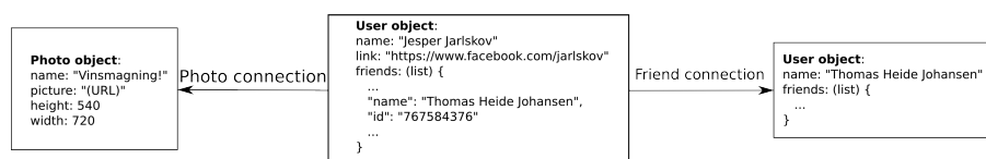
Figure 3.5: Example of a user object in the Facebook Graph API. The User has a connection to a friend represented by another user object, as well as to a photo object.
