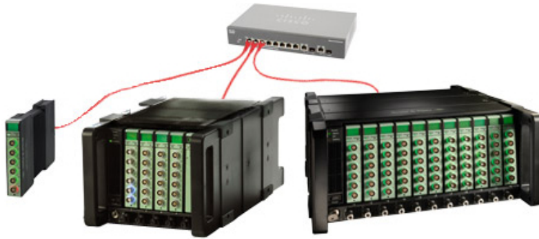
Figure 1.2: A single LAN-XI module, a 5-module frame and an 11-module frame connected to a network switch.
