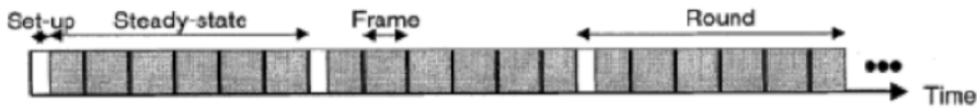
Figure 2.6: Time line showing Leach operation. Adaptive clusters are formed during the setup phase and data transfer occurs during the steady state phase [6]
