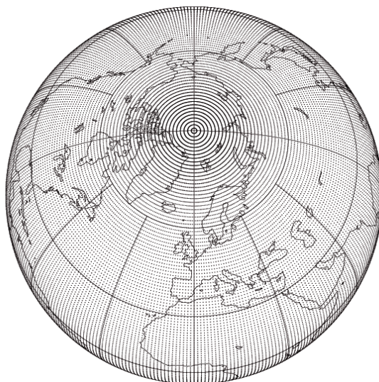
Figure 2.8: Example of a grid of a numerical weather prediction model (source http://rda.ucar.edu )
