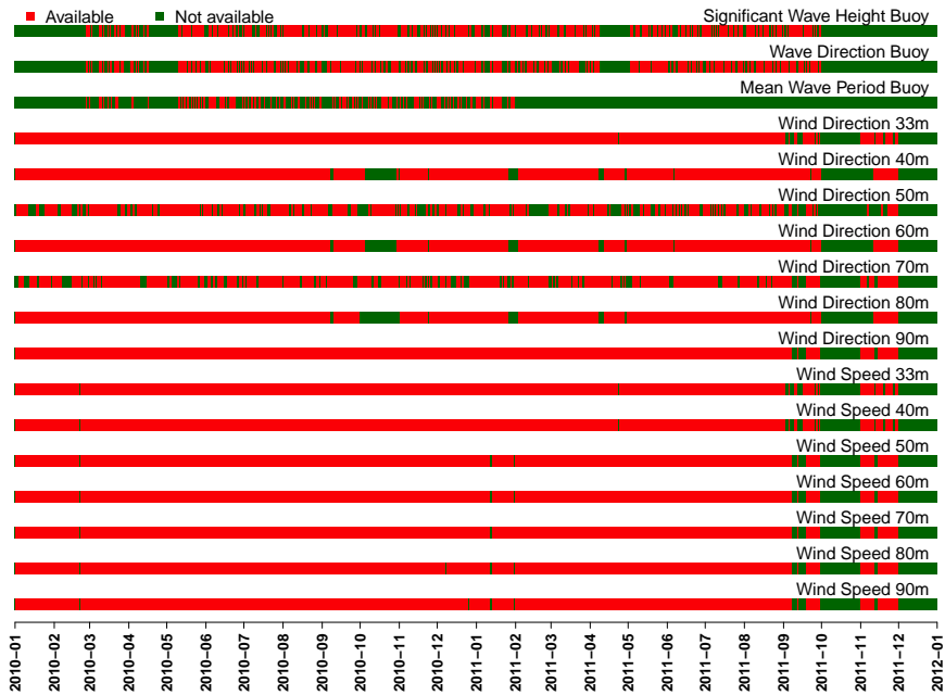
Figure 2.7: FINO_1 mast and buoy measurements availability over 2010-2011 (red symbolizes period when data is available, green symbolizes period when data is missing)
