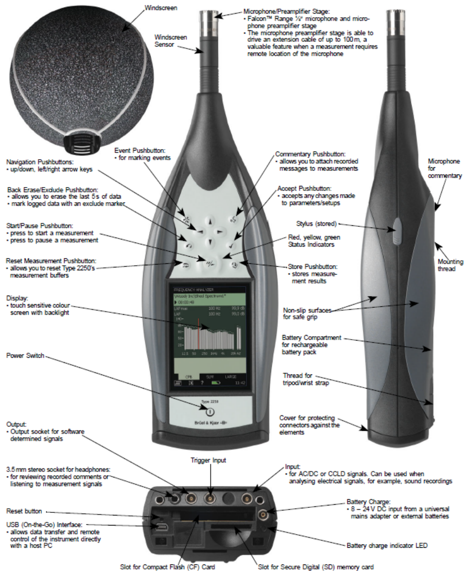
Figure 1.1: Hardware overview of the 2250. Source: [5, p. 4]
