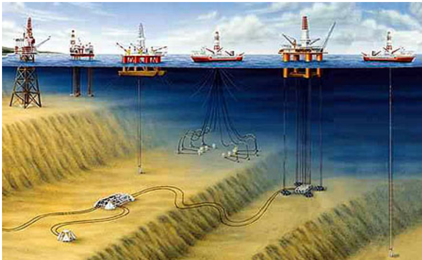
Figure 1.1: A cross-section view of an offshore field equipped in a smart well system driving subsea production [4]
