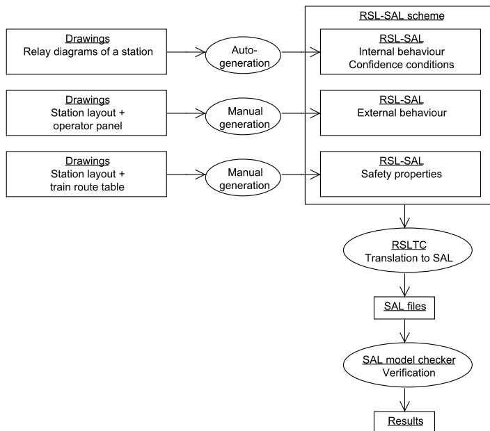
Figure 4.1: The verification method defined by this thesis for checking safety properties of an interlocking system
