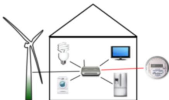
Figure 1: An example of a centralized HAN.
