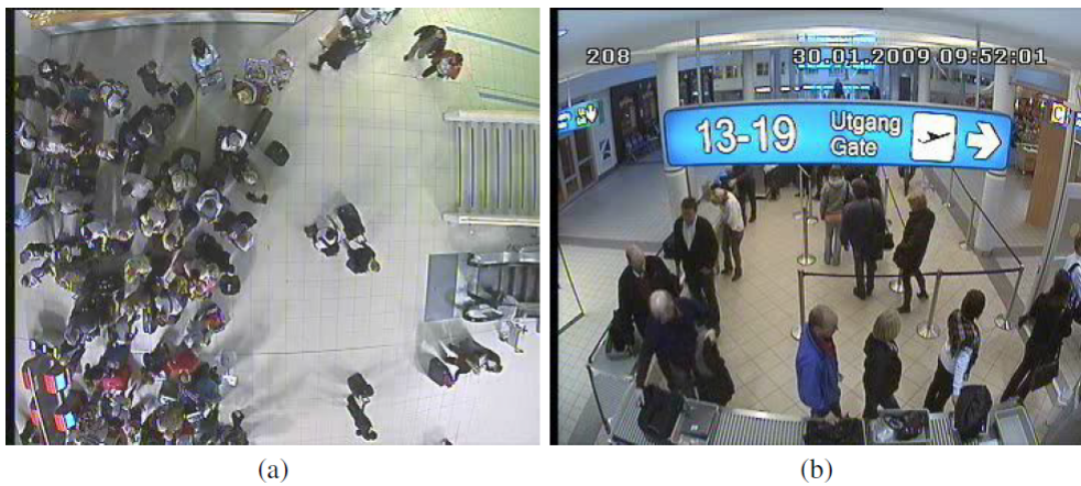
Figure 4.5: High and Low ceiling mounted cameras positions.[VP11]
