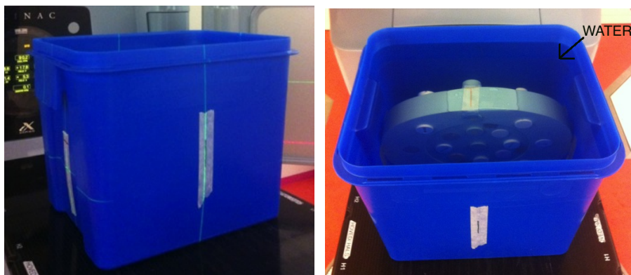
Figure 5.3: (Left) Illustrates the set-up using the laser positioning system. Right) Illustrates the method of scanning PDP in water.
