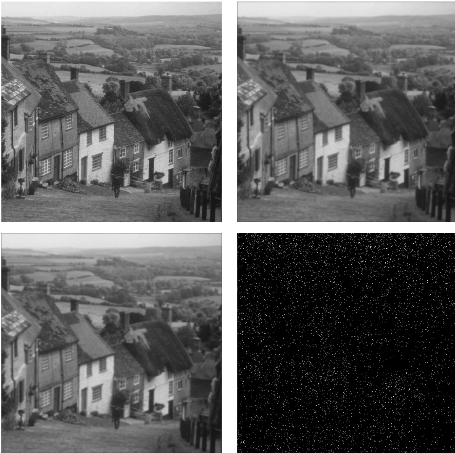
Figure 2.4: Visual result of image smoothing performed by floating point (top right) and integer (bottom left). Original image (top left), Error map of |\bar{\epsilon}|^p between the two (bottom right), magnified 255 times.
