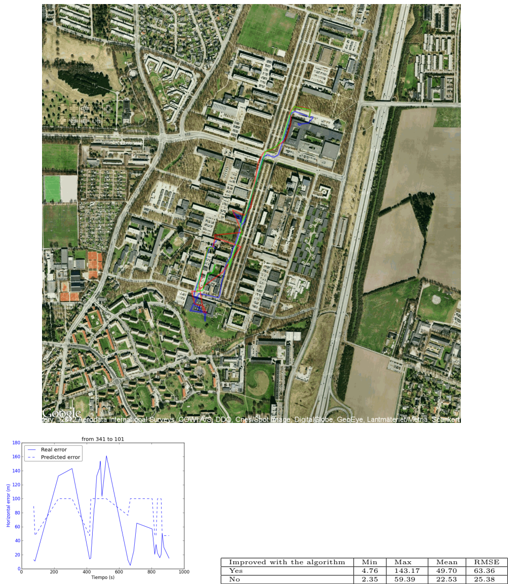
Figure D.2: Route map and error graphs. From 341 to 101
