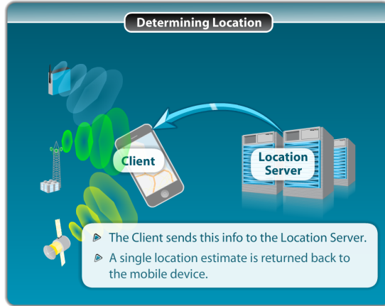
Figure 2.1: Example of hybrid positioning system a
