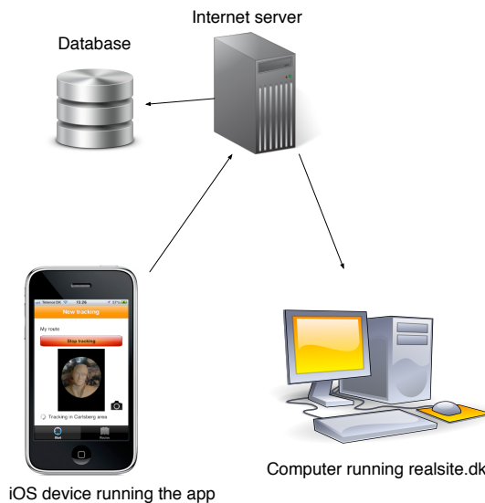
Figure 4.1: System architecture diagram a
