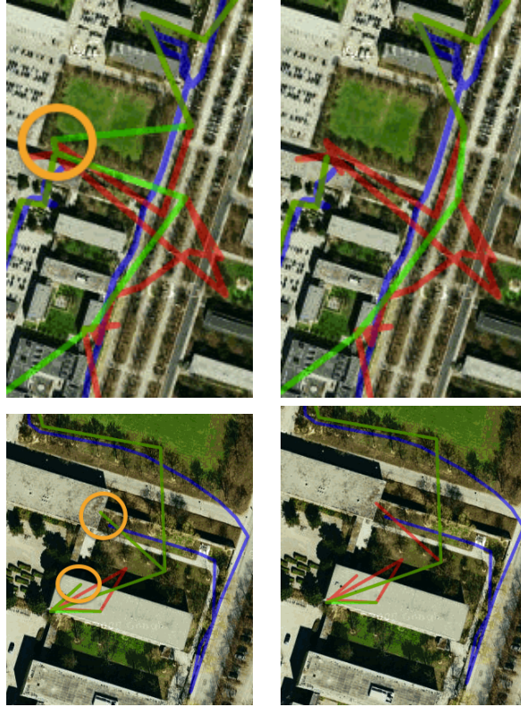
Figure 2.19: Two examples of removing Wi-Fi positions (inside yellow circle) in routes: from 341 to 101 (above) and from 343 to 308 (below)
