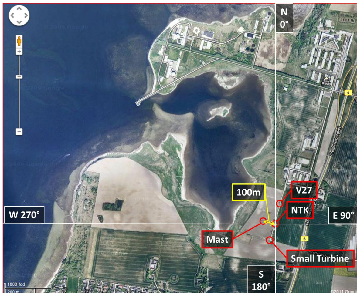
Figure 6 – Risø turbine row and met mast layout
