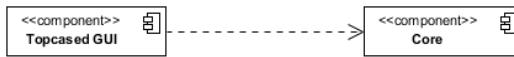
Figure 6.8: EsculapaUML plug-ins. The GUI plug-in depends on core plug-in. The core plug-in does not need the GUI plug-in to work.
