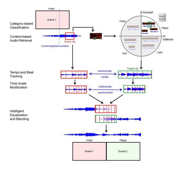
**Figure 12** Possible pipeline for an automated sound track generation system.
