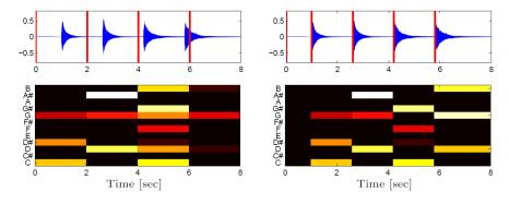
**Figure 6** Waveforms and chroma representations using a fixed-size windowing strategy (left) and an adaptive windowing strategy using beat-synchronized windows (right).
