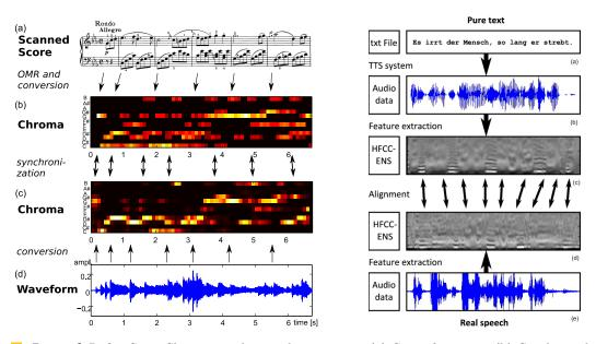
**Figure 6 Left:** Score-Sheet to audio synchronization—(a) Score fragment, (b) Synthesized Chroma features, (c) Chroma obtained from audio recording (d). **Right:** Text to audio synchronization—(a) Text, (b) Synthesized speech, (c) HFCC-ENS features of synthesized speech, (d) HFCC-ENS features of natural speech (e).
