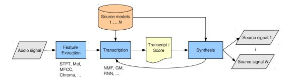
**Figure 1** A unified view on monaural multi-source analysis of speech and music. Spectral (short-time Fourier Transform, STFT) or cepstral features (MFCCs) are extracted from the audio signal, yielding a transcription based on non-negative matrix factorization (NMF), graphical models (GM), recurrent neural networks (RNN) or other machine learning algorithms. The transcription can be used to synthesize signals corresponding to the sources or to enable (more robust) transcription in turn.
