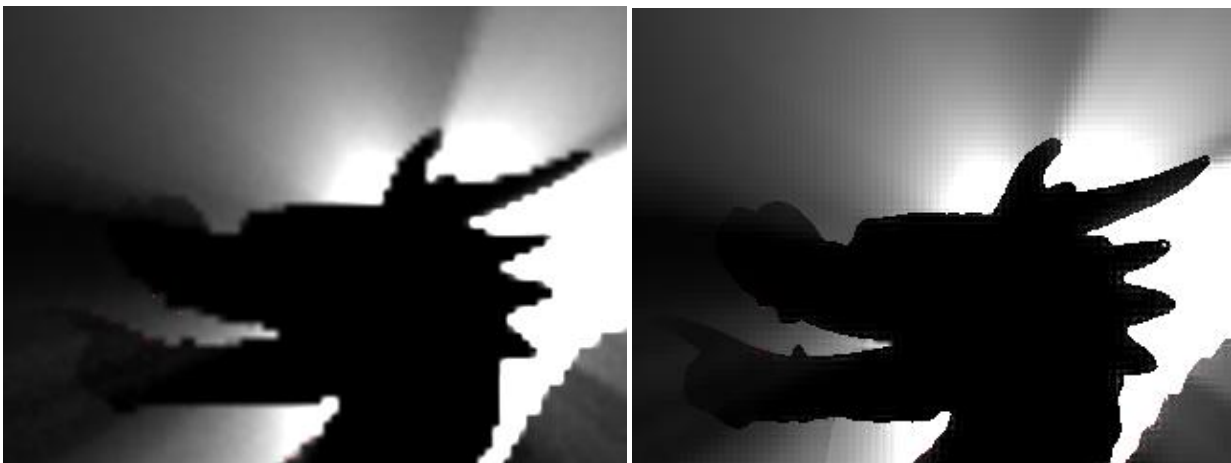
FIGURE 32 - EDGE-ALIASING CAUSED BY LOW RESOLUTION FOG CALCULATIONS WITHOUT UP-SAMPLING (LEFT) AND WITH (RIGHT)
