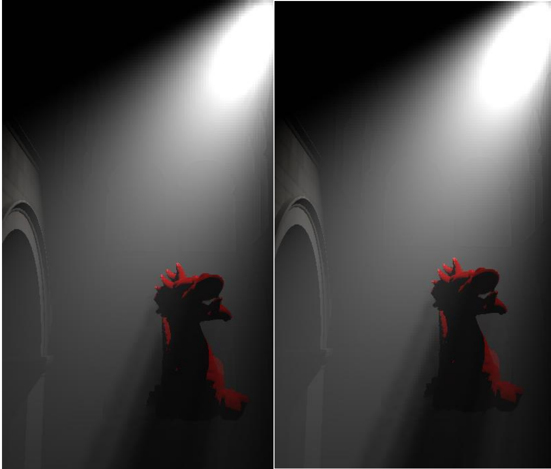
FIGURE 36 - THE SCHLICK PHASE FUNCTION (LEFT) ESTIMATED WITH THE ISOTROPIC PHASE FUNCTION, AND AN 'ARTIST'-MULTIPLIER OF 20
