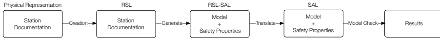
Figure 3.3: The physical representation of the station documentation is manually converted to the RSL representation.
