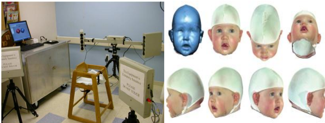
Figure 6: The image to the left shows the 3dMD surface scanner used for acquisition of surfaces of the head (from [5]). The surfaces to the right provide an example of 3dMD surfaces of the head shown in various orientations. The blue surface shows the three-dimensional rendering of a subject scan. The other 7 images show the scan with color texture seen from different perspectives (Modified from [22]).
