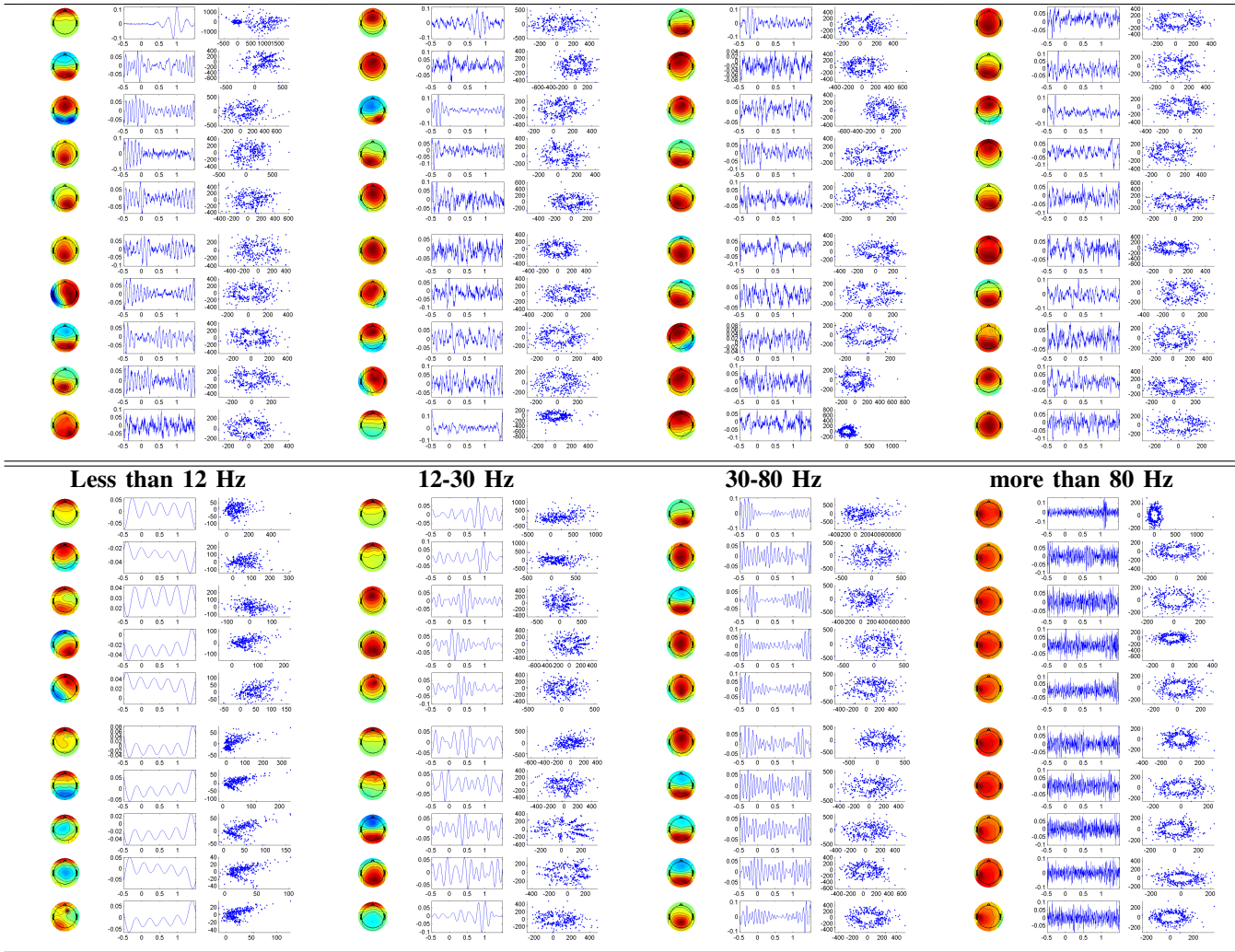
Fig. 2. Top panel: 40 component analysis of the real event related EEG data without frequency constraints. Bottom panel: 40 component analysis of the real event related EEG data with frequency constraints. The delay and trial dependent strength is plotted in a 2D-plane as a complex vector given by c_{k,d} \exp(-i2\pi\tau_{k,d}/T)
