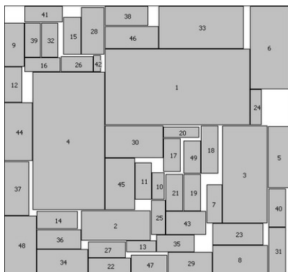
Figure 2.2: Example Floorplan. The grey boxes represent macro blocks while the white boxes is empty unused space, also known as white space (from [22]).
