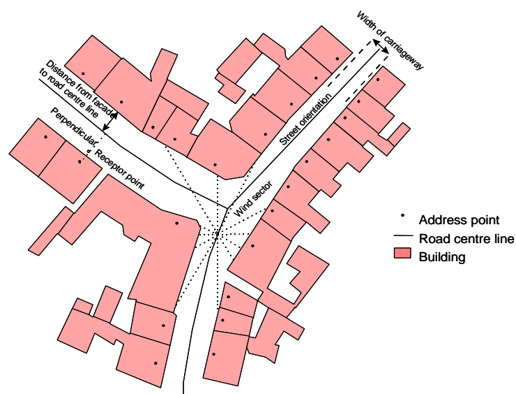
Figure 3: The 2½ dimensional Urban Landscape Model of the AirGIS system that automatically generates required street configuration and traffic input data for the Operational Street Pollution Model (OSPM)
