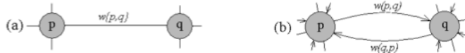
Figure 4.2: (a) Undirected graph: One link from node p to node q. (b) Directed graph: Two links, one from node p to node q and a reverse from node q to node p. The two links can have different capacities [4].
