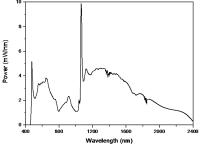
Produces a bright output from 500 nm to 2500 nm, and the beam requires optical filtering to be used in spectral imaging.
