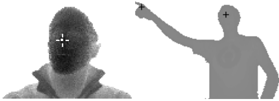
Figure 10: Left: Example nose-detection results shown on ToF range image; detection error rate is 0,03 [HBMB08a]. Right: The direction the user is pointing in can be computed from the difference vector between the positions of the head and hand [HBMB09].
