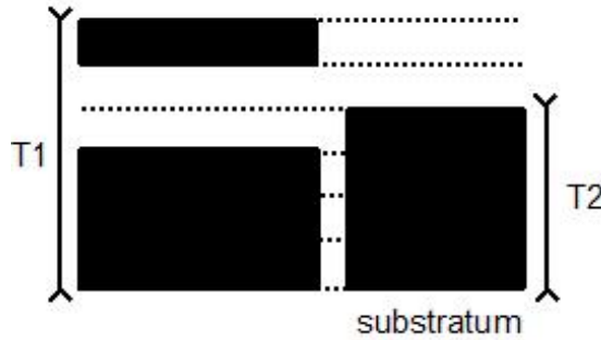
Figure 4.3: Due to the nature of the Maximum Thickness function, the two thicknesses T_1 and T_2 are equal. Only slices with contents are observed.
