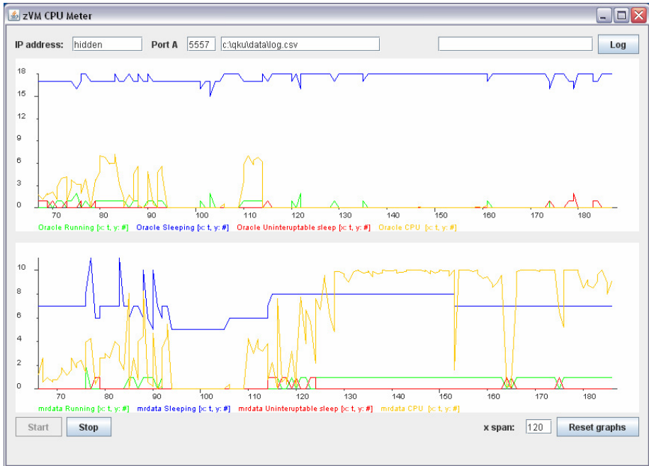
Figure 5-2: The GUI of the developed Java client program, which is used together with the qkumon monitor. (Graphs are based on a class from the JChart2D library from http://jchart2d.sourceforge.net .)
