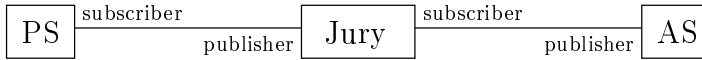
Figure 5.2: The Publish-Subscribe architecture: Jury acts as a subscription agent between AS and PS systems, i.e., it receives AS messages on behalf of protected systems.
