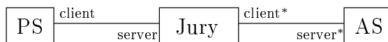
Figure 5.1: The Client-Server architecture, the connections between the Jury framework and remote AS nodes are marked with a star because although they act like a client-server, the AS is responsible for initiating the connection.
