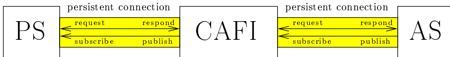
Figure 5.3: All messages between a remote system and the CAFI are sent using the same persistent connection, regardless of whether they are request/response messages or event notifications.
