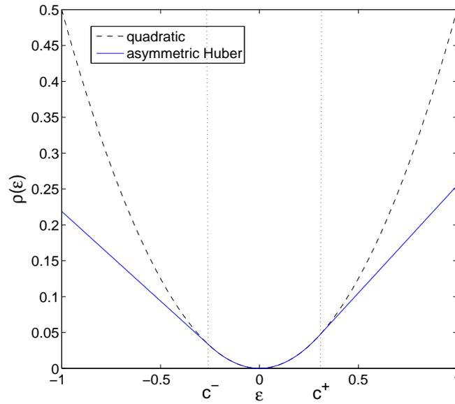
Figure 9: The ‘usual’ quadratic ( $\rho$ ) and asymmetric Huber ( $\rho^\dagger$ ) criterion functions. The thresholds points  $c^-$  and  $c^+$  locate the negative and positive transitions from quadratic to linear criteria. Here these points are such that  $c^- = -0.25$  and  $c^+ = 0.3$ . Negative residuals larger than  $c^-$  (in absolute value) and positive residual larger than  $c^+$  are then downweighted when updating the model estimates.
