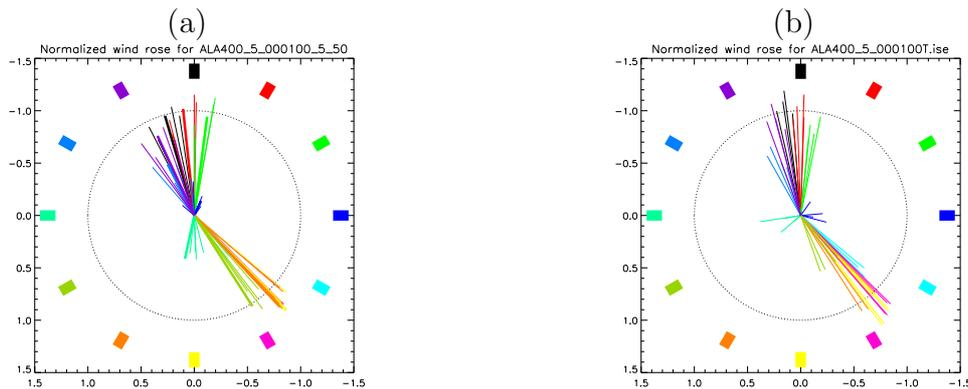
Figure 5: Diagrams showing the mesoscale effects on the geostrophic wind forcings from 12 directions using the  $10 \text{ ms}^{-1}$  and typical stability profile given by (a) KAMM and (b) WRF. Each set is made up of 12 simulations using different wind directions indicated by the colours. Please refer to the main text for an explanation of the figures.
