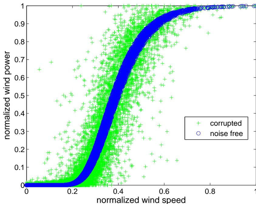
Figure 10: Noise-free and corrupted power curves.
