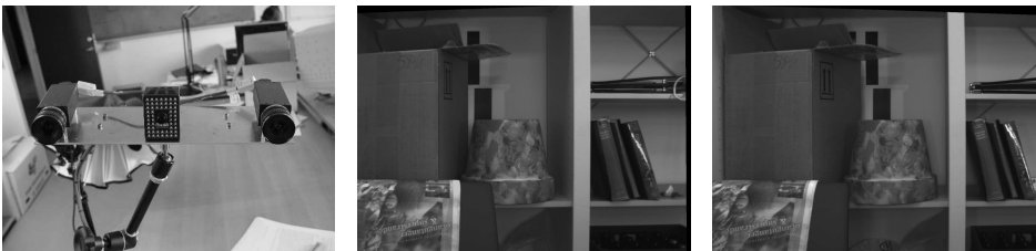
Figure 2 The TOF-Stereo rig and the rectified image pair used in the experiment.
