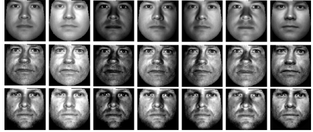
Figure 5. Face re-lighting using combined model. Each row contains synthesized images that belong to the same identity. Images at each row are synthesized by changing illumination parameters in the AIA Model for the same identity.
