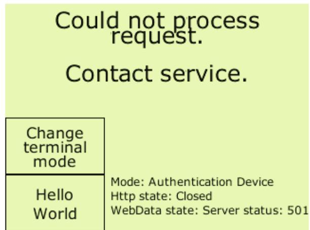
**Figure 17-9** The authentication device could not reach the server.
