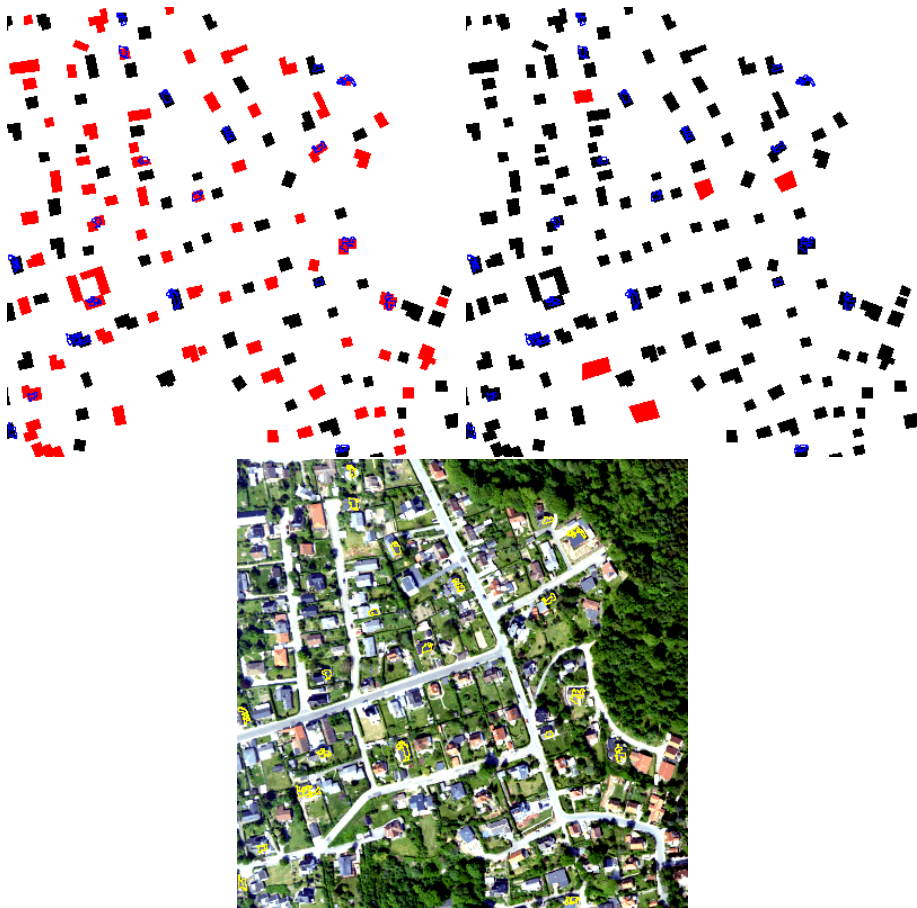
Figure 6.20: Test area 2 MLE, UL: Detection of new buildings, UR: Detection of demolished buildings, LC: Vectorized building clusters on RGB image.
