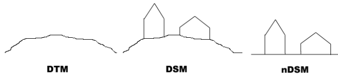
Figure 2.16: Principle of the nDSM in profile.
