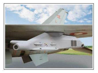
Figure 2.9: A pylon mounted under the wing. IR sensors are placed in the front and the back of the pylon. The holes on the rear end of the pylon will contain chaff or flare cartridges to be dispensed during flight. (Photo courtesy of Terma.)
