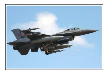
Figure 2.8: Bombs and missiles mounted at stations underneath an F-16 fighter aircraft. (Photo courtesy of Erwin Stam.)
