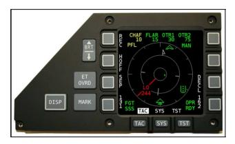
Figure 2.6: An azimuth indicator as part of the Advanced Threat Display. (Photo courtesy of Terma.)
