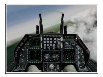
Figure 2.10: The cockpit of an F-16 fighter aircraft. Above the knees of the pilot two MFDs can be seen. The azimuth indicator is positioned to the top left, above the left MFD. (Screenshot from the Falcon 4.0 flight simulator from Microprose.)
