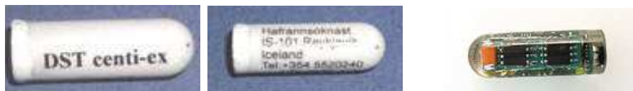
Figure 5.2: Various types of DSTs used for geolocation. Left: Star-oddi centi, Center: Star-oddi milli, Right: LTD 1110 (similar to 1200).
