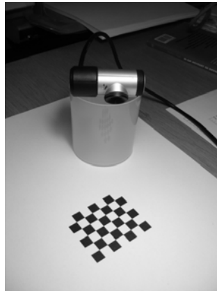
Figure 5.26 The setup used to calibrate the camera
