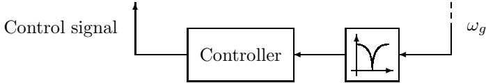
Figure 3.7: The hybrid controller setup is stabilised by bandstop-filtering the generator speed signal before the controllers.
