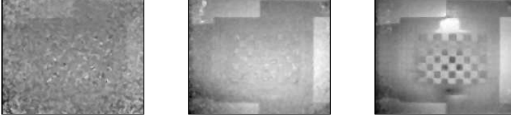
Figure 2.5: Changing the Integration Time. The integration time set to 1 msec, 10 msec (auto), and 25 msec , the measured distance in the center pixel is also given.
