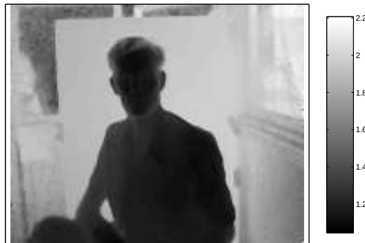
Figure 1.1: A Range Image . The dark regions are close and the lighter are further away. The scale is in meters. The background wall is past the non-ambiguity range and therefore appears 7.5m closer. (Captured with the Swiss-Ranger)
