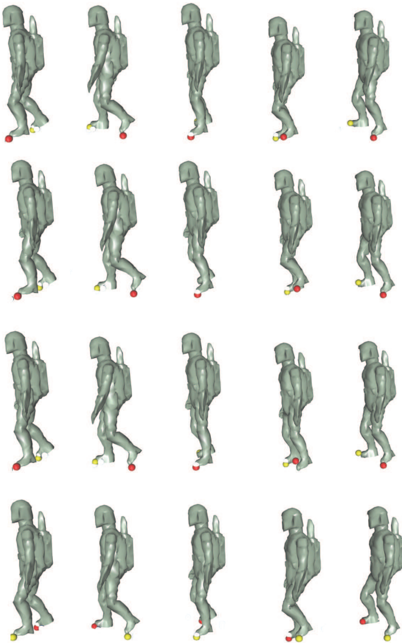
Figure F.2: Poses from walk animation using DtT+DfE on example set A. From top down: 1) Simple Hill Climbing. 2) Hooke and Jeeves. 3) Simple Hooke. 4) Global exhaustive.
