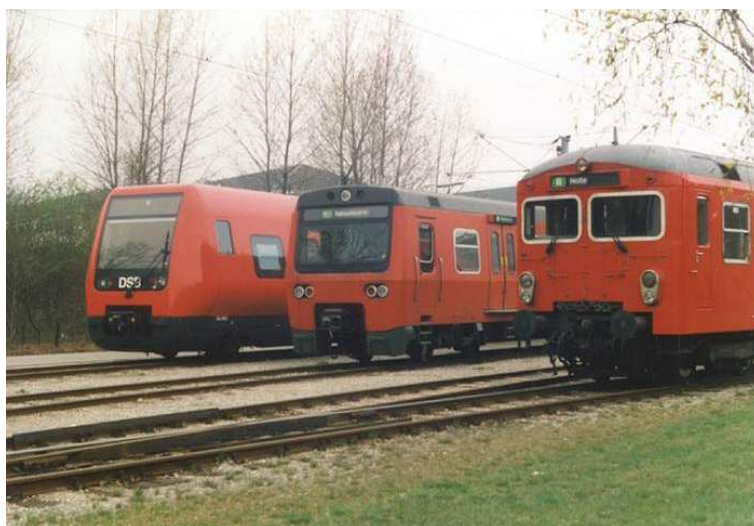
Figure 3.4: Three generations. To the left a 4th generation S-train, in the middle a 3rd generation S-train and to the right a 2nd generation S-train [Chr06].
