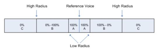
Figure 13: How the score is calculated. If a vocal falls in zone A it gets 100%, zone B is linear from 0-100% depending on how close to A it is and zone C gives 0%
