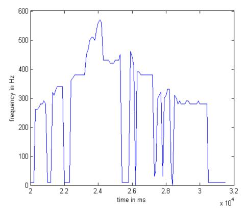
Figure 6: The most powerful frequency, calculated with FFT, on an recorded vocal, same time period as in Figure 8-12. We used 100ms non-overlapping windows. The graph looks much better than figure 4 for using as a basis for our calculations.
