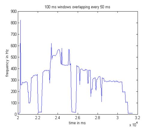
Figure 11: Most powerful frequency, calculated with FFT with 100 ms windows and with 20 samples per second.
