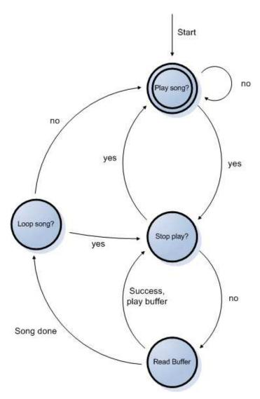
Figure 3: Figure 3: State chart for song playing in SoundThread class. It supports play, stop and looping songs
