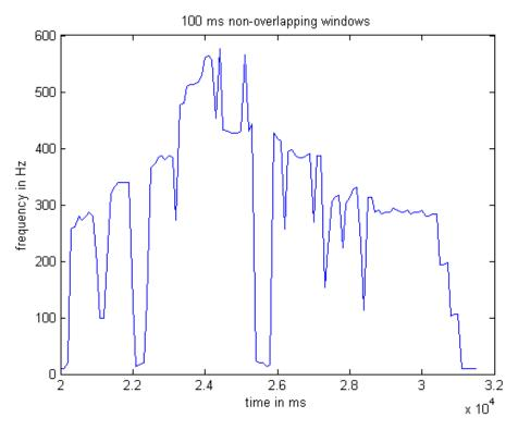
Figure 12: FFT with 100 ms windows and 10 samples per second
