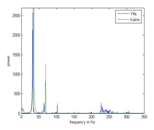
Figure 7: Comparing power of frequencies of two recordings. Both have a maximum at around 35 Hz which means our algorithm works for these two vocals.
