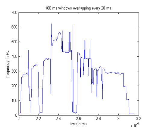
Figure 10: Most powerful frequency, calculated with FFT with 100 ms overlapping windows and with 50 samples per second.
