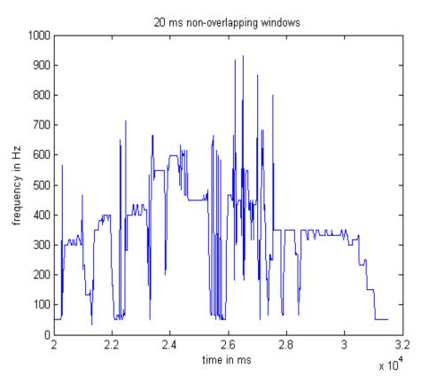
Figure 9: Most powerful frequency, calculated with FFT with 20 ms windows and with 50 samples per second.
