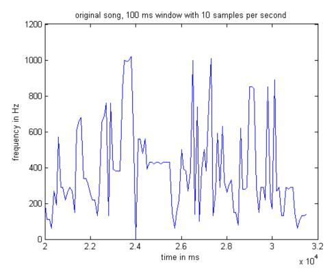
Figure 4: The most powerful frequency, calculated with FFT, on an original track with vocals and instruments, same time period as in Figure 8-12. We used 100ms non-overlapping windows. The graph has too many spikes and rapid changes to use.
