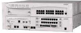
Figure 9.4: Avaya ISTS IP PBX which can be made by a Media Gateway G650 and a Media Server S8700.
